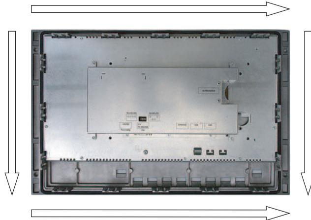
The following table shows the positioning of the mounting clamps on the MP 277 10" Key. Observe the counting direction. The position indicated corresponds to the first recess occupied for each mounting clamp in the counting direction. The inserted mounting clamp covers two recesses.
