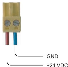
Connect the power supply cables to the terminal block as shown in the figure above. Ensure that the lines are connected properly to the correct terminals. Refer to the label for the contact pins on the rear of the HMI device.
