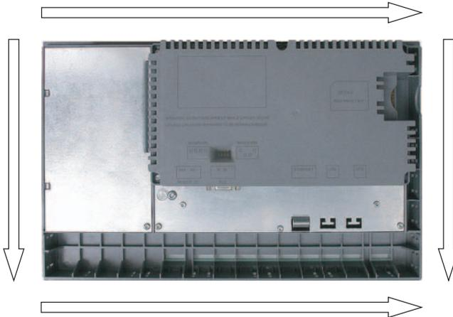
The following table shows the positioning of the mounting clamps on the MP 277 8" Key. Observe the counting direction. The position indicated corresponds to the first recess occupied for each mounting clamp in the counting direction. The inserted mounting clamp covers several recesses.
