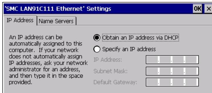
2. Select either automatic address assignment via DHCP or manual address assignment.
