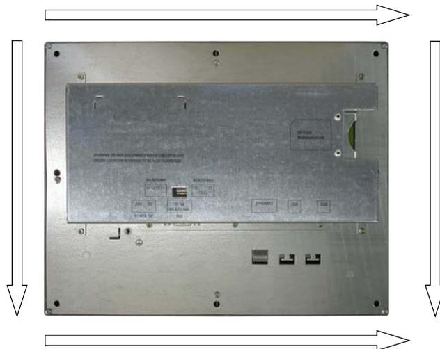
The following table shows the positioning of the mounting clamps on the MP 277 10" Touch. Observe the counting direction. The position indicated corresponds to the first recess occupied for each mounting clamp in the counting direction. With the MP 277 10" Touch, you can only use every other recess to attach the mounting clamp. Only those recesses were counted, which a mounting clamp can be used for. The inserted mounting clamp covers several recesses.
