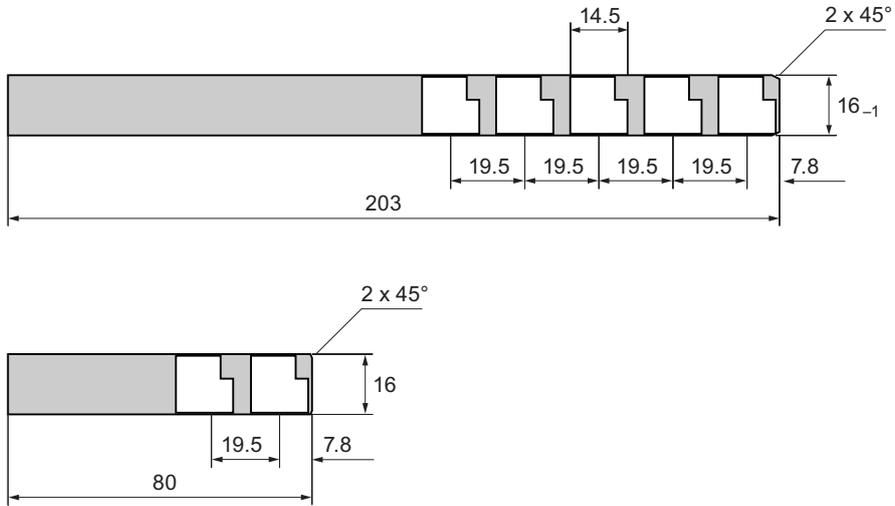
Dimensions of the labeling strip for the MP 277 10" Key
