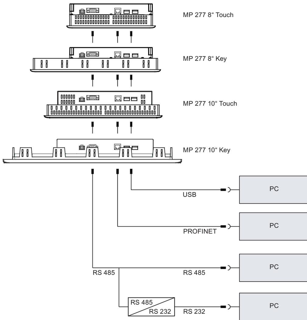
Use a cross-cable for the PROFINET connection when using a point-to-point connection.
