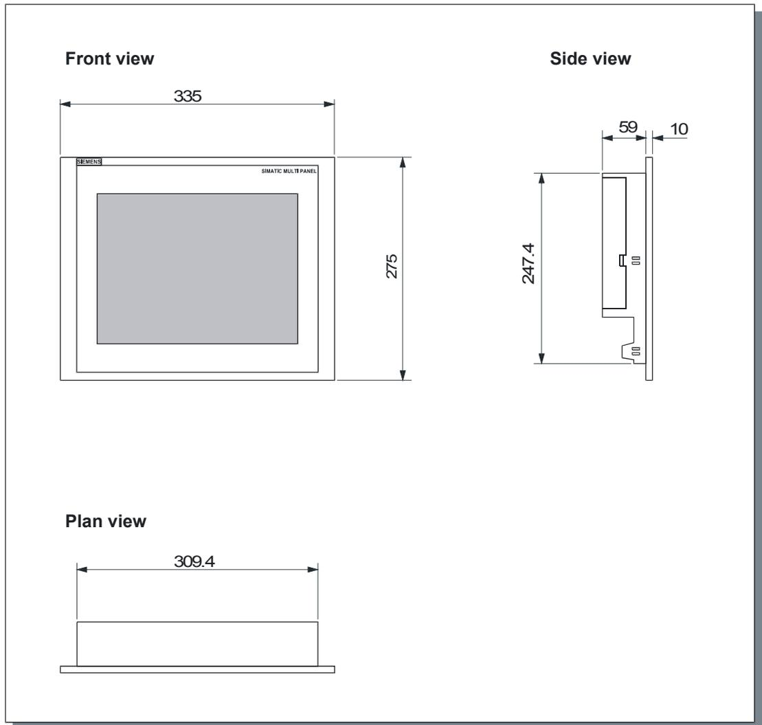
Figure 12-1 Dimensions of the MP 370 12" Touch
