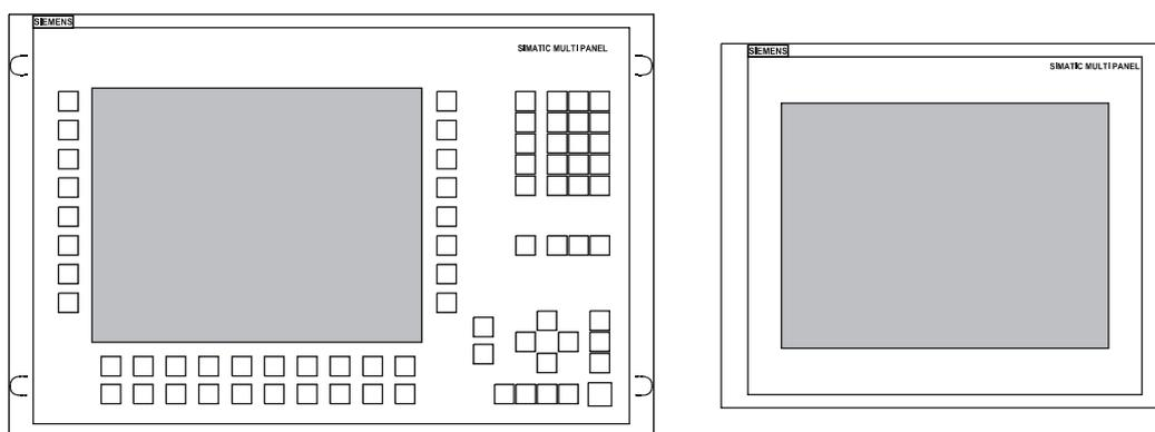
Figure 1-2 MP 370 as keyboard unit and touch panel unit
