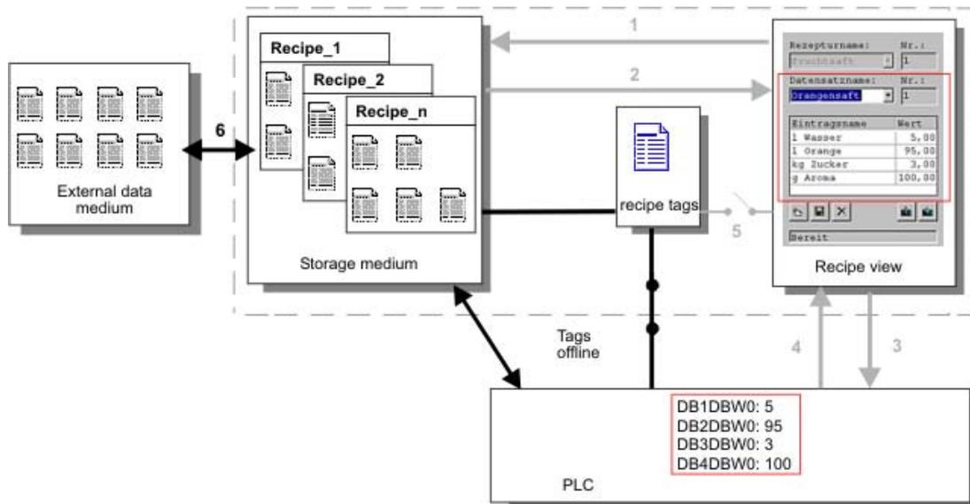
Production can be controlled using one or more "Scripts", which transfer production data records automatically to the PLC. The sequence can be checked using the return values of the utilized functions.
