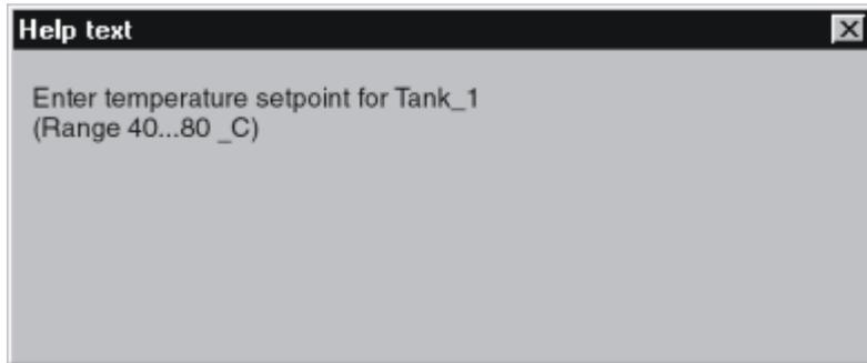
Figure 9-4 Operator note for an I/O field (Example)
