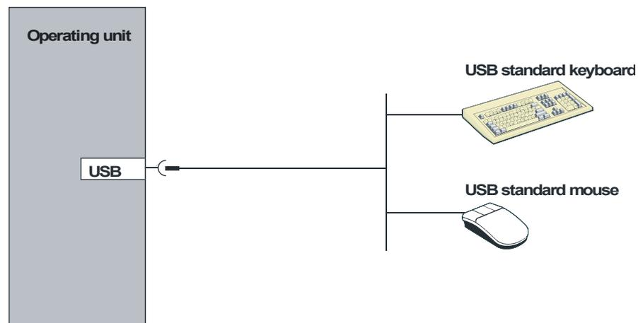
Figure 4-6 Connection configuration for external keyboard and mouse
