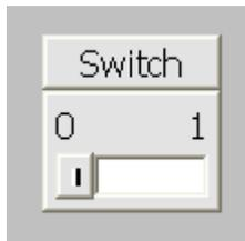
A switch has two stable states: When you actuate the switch, it changes to the other state. The switch retains this status until the next operation.
