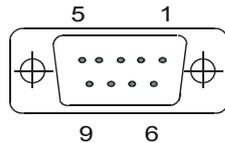
Table 12-2 9-pin Sub-D socket (configuration via switch)
