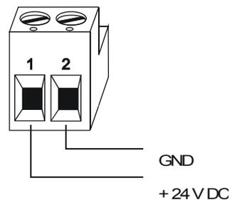
Ensure that the lines are connected properly to the correct terminals. Also note the labeling for the contact pins on the back of the HMI device.
