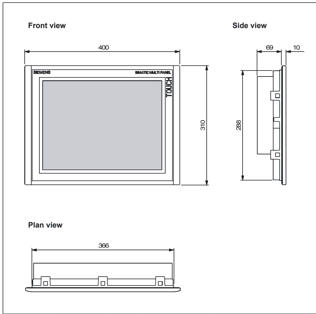
Figure 12-2 Dimensions of the MP 370 15" Touch
