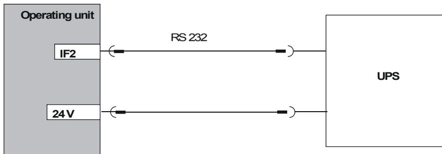
Figure 4-9 Connection configuration for an uninterruptible power supply
