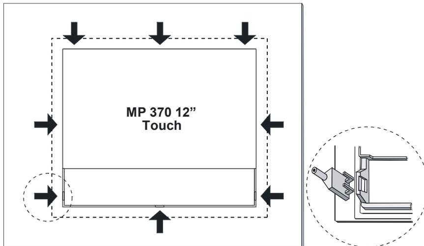
Figure 4-1 Screw clamps on the MP 370 12" Touch
