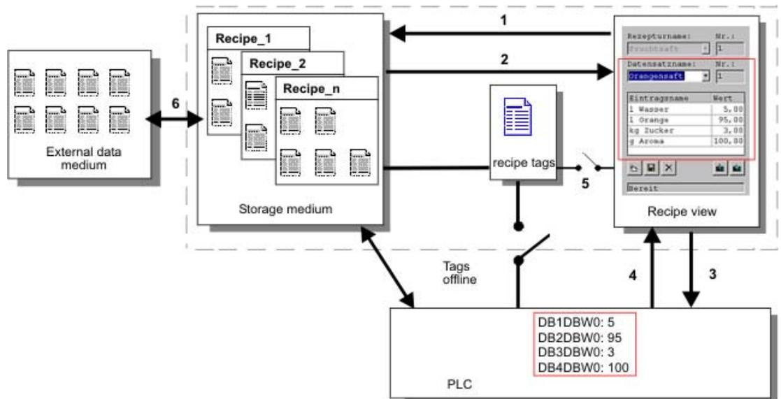
The HMI device stores recipe data records on a storage medium such as a flash memory device or hard disk. You can edit a recipe data record in a recipe view or recipe screen on the HMI device display.
