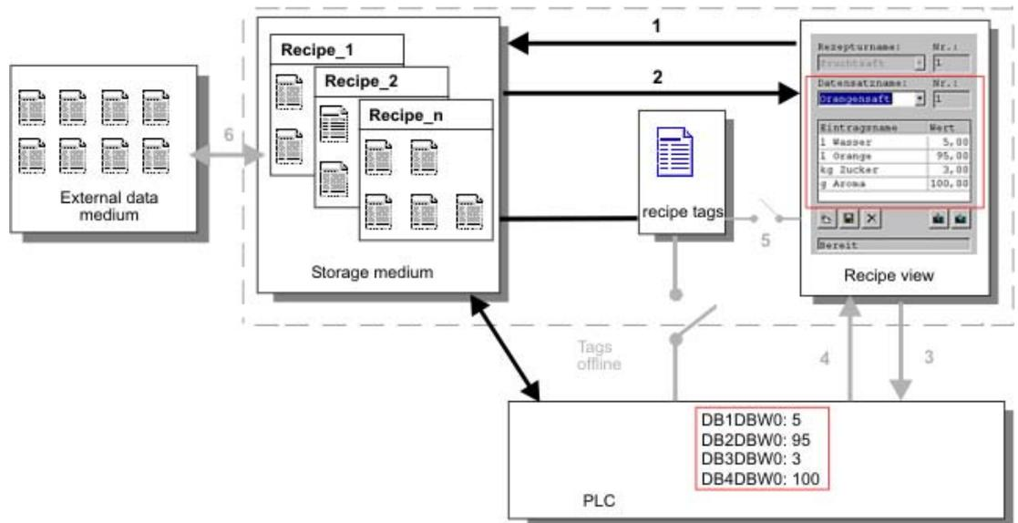
You enter the production data in the recipe view or the recipe screen, assign a recipe data record name, and save the new recipe data record on the storage medium of the HMI device.
