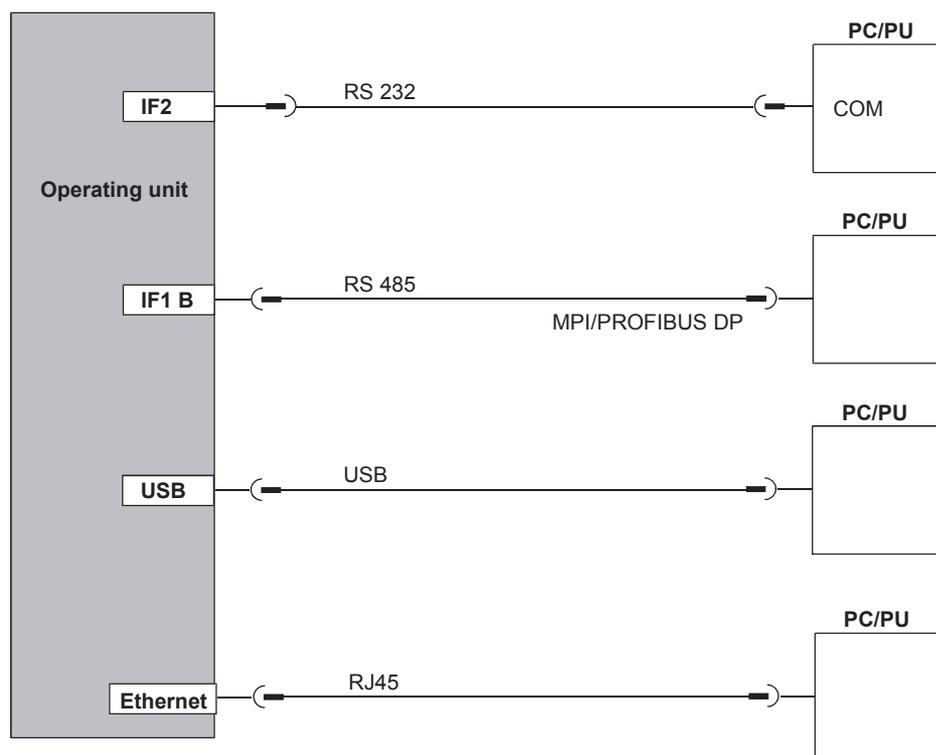
Figure 4-8 Connection configuration for configuration computer
