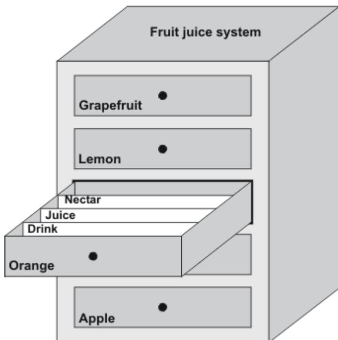
A recipe data record is a set of values for the tags defined in the recipe. You enter the values in the input fields. You can enter the values either during configuration or during runtime on the HMI device or the machine.
