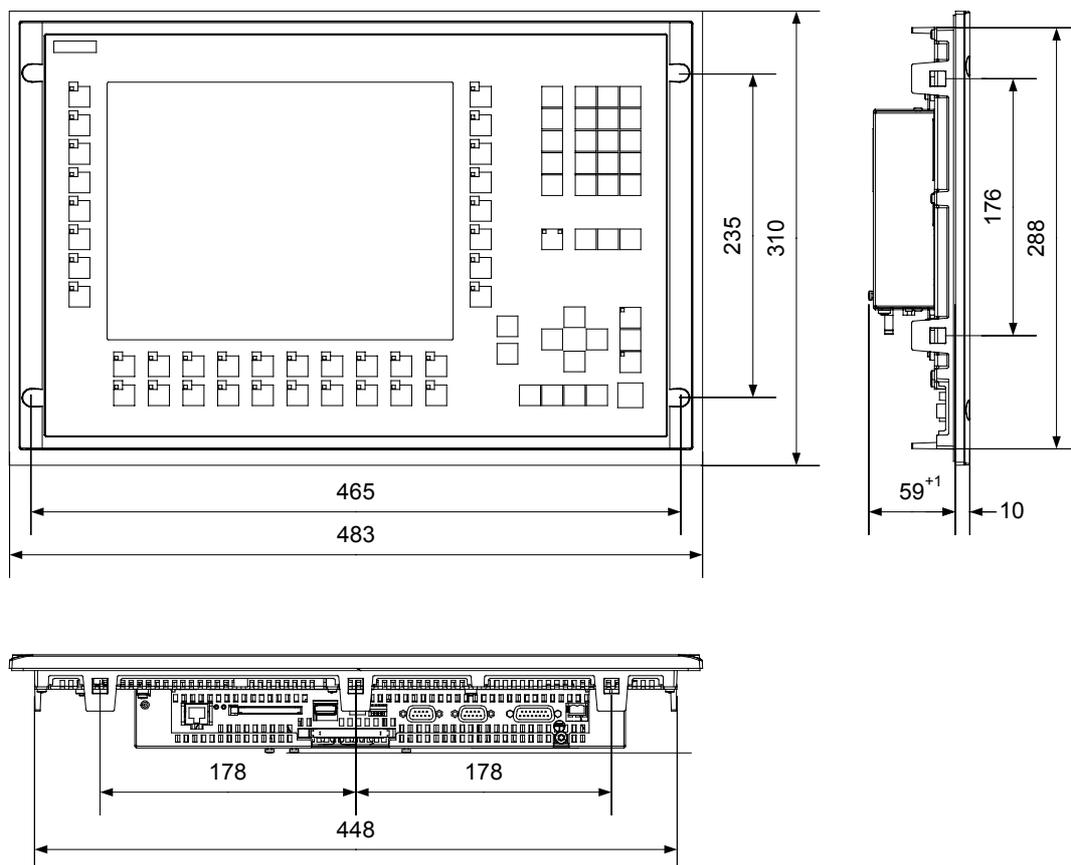
Figure 12-3 Dimensions of the MP 370 12" Key
